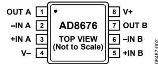
Figure 2. 8-Lead MSOP (RM-8)
