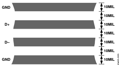
Figure 20. Arrangement of Signal Tracks
